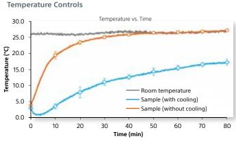
The graph describes the impact of the cooling plate on sample temperature during an 80-minute plate acquisition.
