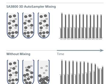
This figure illustrates how cell heterogeneity is maintained using the system's 3D mixing function. Without mixing, larger cells settle to form heterogeneous samples, as shown in the lower illustration. Graph data describes how the sample integrity is maintained throughout plate acquisition of 3-µm and 10-µm beads from wells 1–96 to deliver more complete, consistent results.
