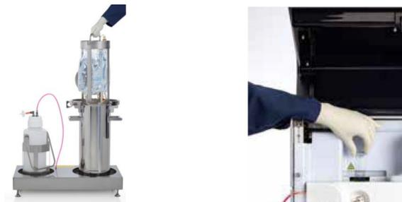
Figure 4: FX500 sheath tank with sheath rack and saline bags
