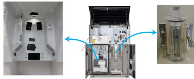
Figure 5: FX500 sort collection area and sample loading chamber
